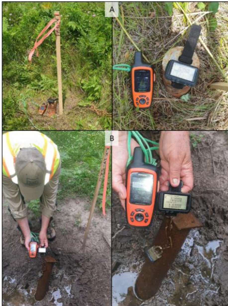
Figure 12-2: Examples of Onsite Collar Location Verifications
