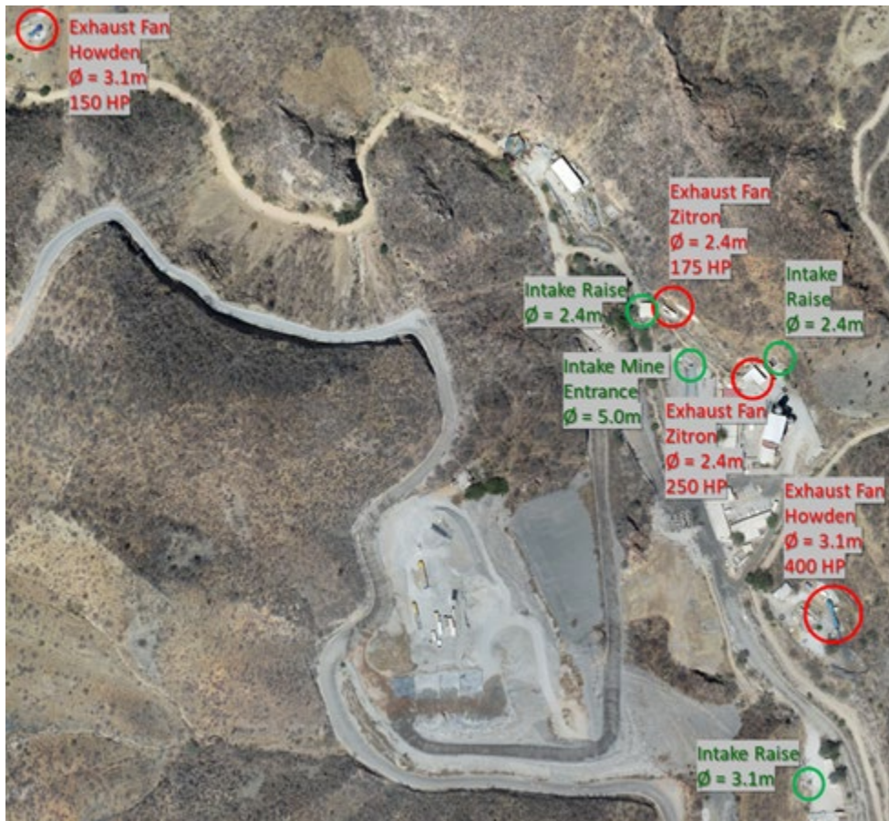
Figure 16-6: Ventilation Fans and Raise Bore Holes Installed at the Arista Underground Mine
